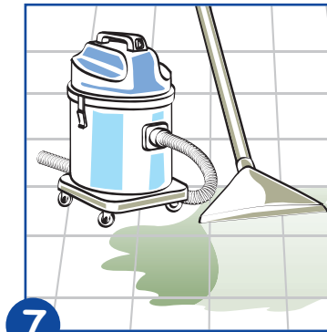
7 Remove slurry with wet suction machine or mop.
